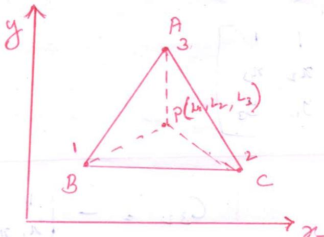
Q1. Consider a triangular element having 3 nodes as shown in fig. If P be a point inside the element as it has 3. Corrdn  $l_1, l_2 \& l_3$
