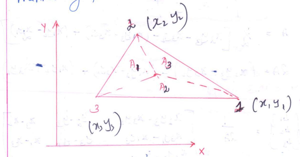
Considering a linear displacement variation of a triangular element is shown in above fig.
